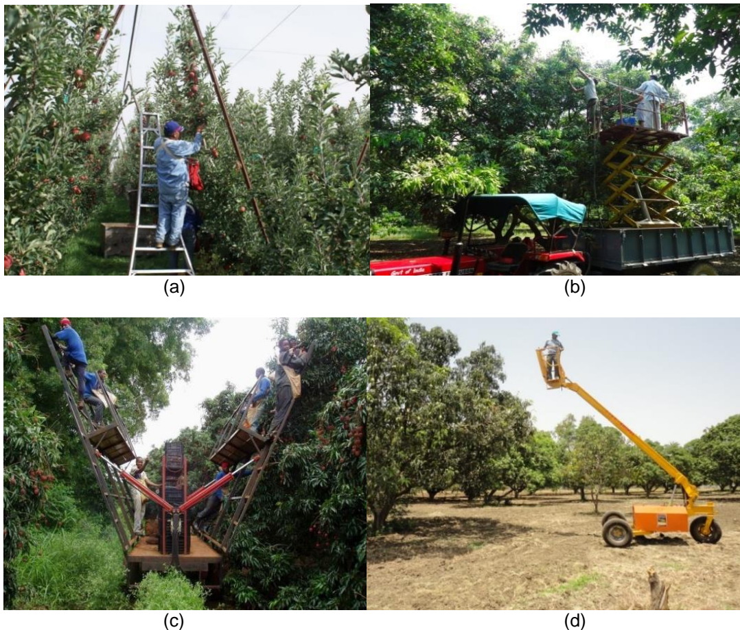
Fig. 11. Harvesting aid for litchi (a) harvesting ladders, (b) tractor-operated hydraulic platform, (c) hydraulic operated ladder, and (d) self-propelled hydraulic platform
