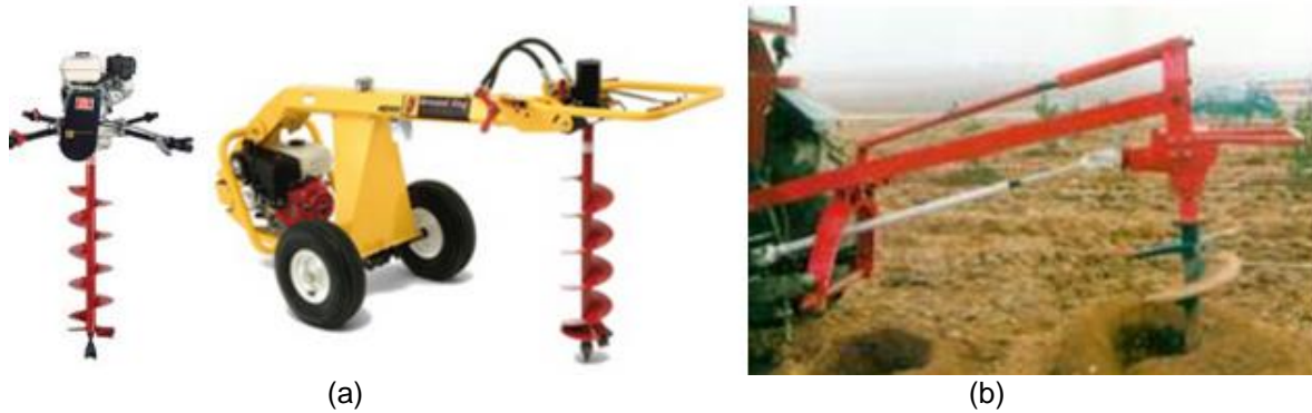
Fig. 4. Pit hole diggers (a) motorized and (b) tractor-operated for digging pits for litchi planting
