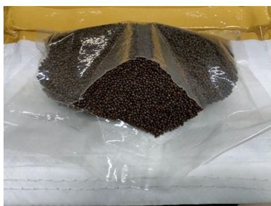
Best results were observed in PP woven Bag with Liner IV (PA/EVOH/PE – 9 Ply; 70-80 \mu )
